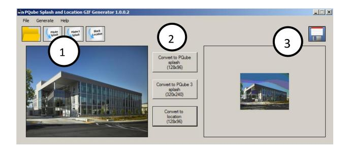
So, no more hassle to scale or modify color palettes with photo edit tools! Open, convert, save it to your SDCard (PQube) or USB thumb drive (PQube 3), insert the card/drive, restart the PQube, and you are done!
