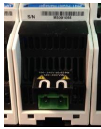
PM1/PM2 rear view— 100 to 240 Vac input terminals
