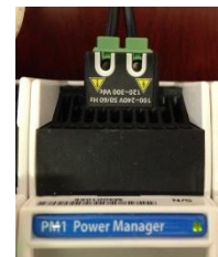
PM1 top view— 100 to 240 Vac input terminals
